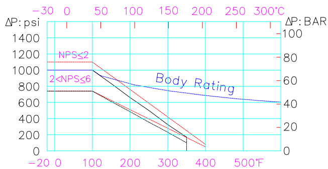
PTFE/R.PTFE Ball SEAT Pressure-Temperature RATING
